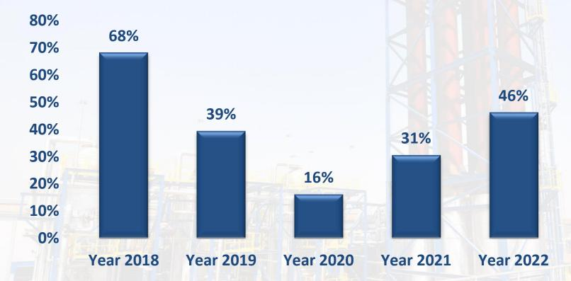
The plant operated at average capacity factor of 794GWh:46.42% (2021: 523GWh :30.59%) during the year. Recovery has been observed due to international issues with RLNG/COAL.
